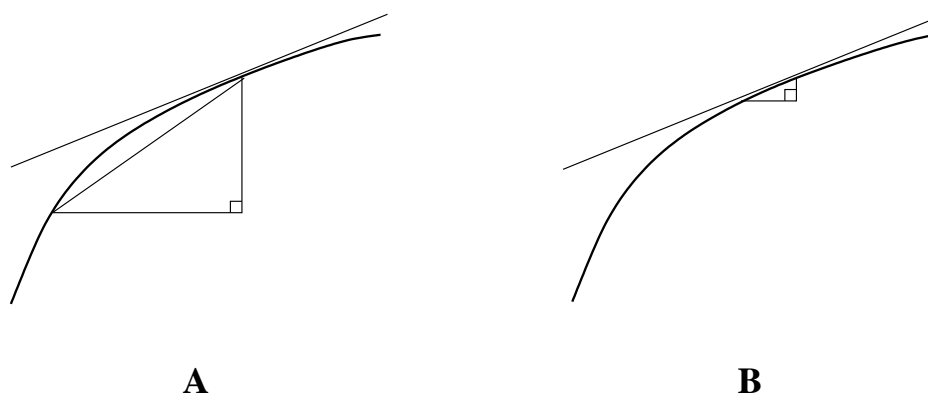
Figure 5.8: Characteristic Triangle. (A) The slope of the tangent at a point is approximated by the hypotenuse of a triangle at that point. (B) The exact slope is given by the infinitesimal characteristic triangle, which has shape but no size.
