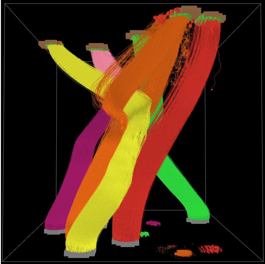
Figure 1.2 Simulation of fiber bundle routing. Six paths (colored arbitrarily for clarity) are created sequentially between randomly chosen origins on the lower surface and randomly chosen destinations on the upper surface. Each path is created by a cohort of 5 000 agents, which together create a bundle of 5 000 fibers. Notice how the orange bundle had to split to find its way past the yellow bundle. As a result, several agents lost their way (one can be viewed near the righthand surface). Small spheres on the upper surface indicate incorrect connections; in this example, there were 162 incorrect out of 30 000 (99.5 per cent correct).
