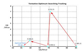
Figure 7. Searching path of the tentative optimum for the 9-bus system.
