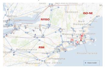
Figure 6. Part of the NPCC system and the most severe N-1 contingency and three candidate buses for dynamic var sources.
