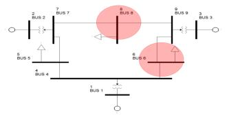
Figure 5. The 9-bus system with the most severe N-1 contingency and two candidate buses for dynamic var supports.
