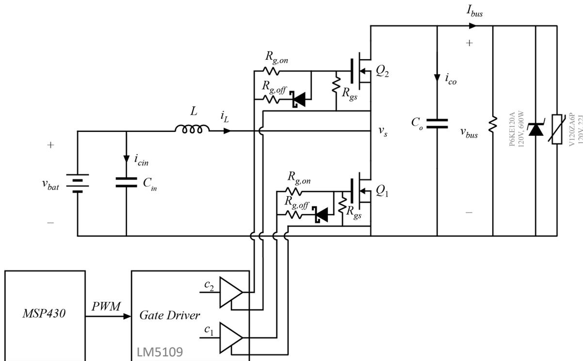
**Figure 1:** Boost converter open-loop power stage schematic
