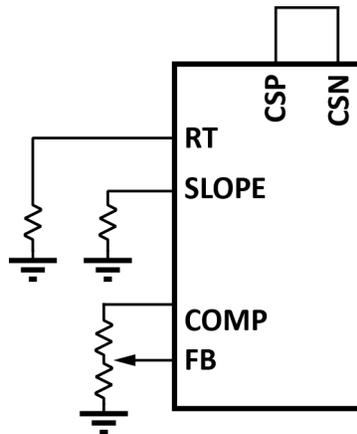
**Figure 2:** Open-loop duty-cycle controlled modulator connections.
