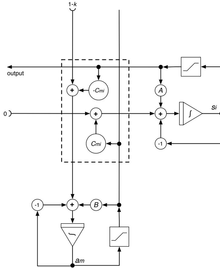
**Fig. 1** Example analog algorithm implementing a dynamical system Boolean satisfiability [12]. The block enclosed in dotted lines is repeated for  $m = 1, \dots, M$  and  $i = 1, \dots, N$ .
