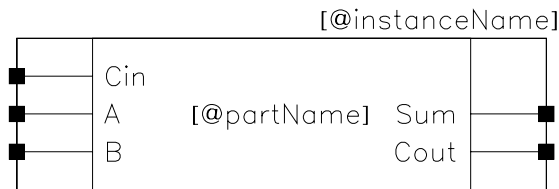
Figure 3.8: A simple symbol for the FullAdder circuit
