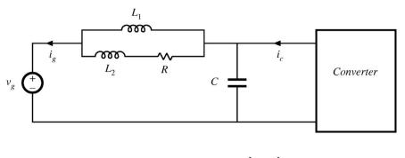
$$G(s) = \frac{i_g(s)}{i_c(s)} = \frac{1 + s \frac{L_1 + L_2}{R}}{1 + s \frac{L_1 + L_2}{R} + s^2 L_1 C + s^3 \frac{L_1 L_2 C}{R}}$$
