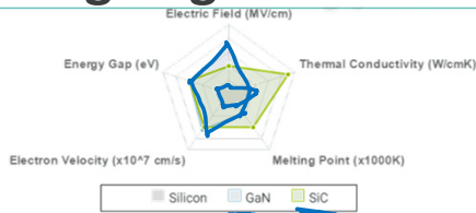
Fig. 1: Material properties of silicon, silicon carbide, and gallium nitride.
