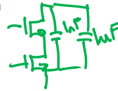
Fig. 8. Paralleled capacitors minimize impedance over frequency.
