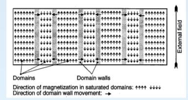
• Therefore, core loss should be directly related to the remagnetization velocity, *dM/dt*, rather than the excitation frequency, *f*.
