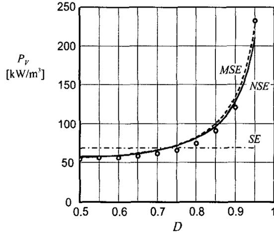
Fig.5 Specific ferrite core losses with square voltage waveforms for ferrite grade 3F3 at 100 kHz, 100°C, 0.1 T as a function of duty ratio  $D$ ; the experiments are the circles; the Natural Steinmetz Extension is the solid curve (NSE), for  $\alpha=1.842$ ;  $\beta=3.06$ ; the Modified Steinmetz Equation (5) is the dashed curve (MSE); classical Steinmetz Equation (1) is dash-dot curve (SE).
