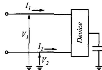
Fig.1 Two wire method. Measuring power to a device with two feeding wires and a ground plane.
