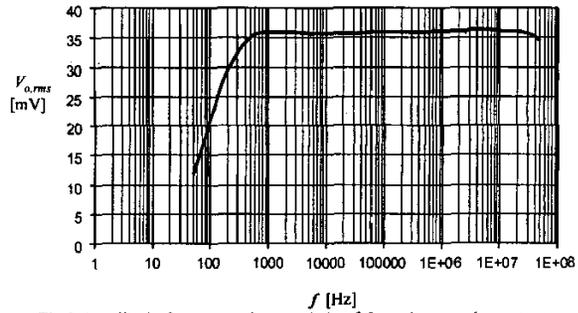
Fig.3 Amplitude-frequency characteristic of the voltage probe, output  $V_{o,rms}=35.36$  mV for 5V sine wave input voltage.
