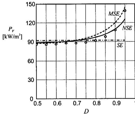
Fig.7 Specific ferrite core losses with square voltage waveforms for ferrite grade 3F3 at 25 kHz, 100°C, 0.2 T as a function of duty ratio  $D$ ; the experiments are the circles; the Natural Steinmetz Extension is the solid curve (NSE), for  $\alpha=1.31$ ;  $\beta=2.9$ ; the Modified Steinmetz Equation (5) is the dashed curve (MSE); classical Steinmetz Equation (1) is dash-dot curve (SE).
