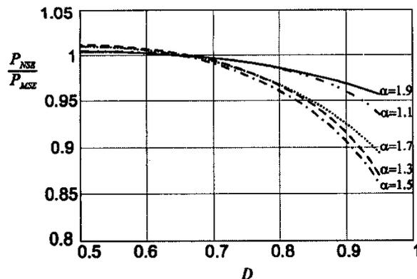
Fig.8 Comparison between NSE and MSE as a function of the duty ratio  $D$ , for different values of  $\alpha$ .
