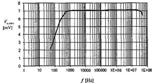
Fig.2 Amplitude-frequency characteristic of the current probe, output  $V_{o,rms}=7.071$  mV for 100 mA peak sine wave input.
