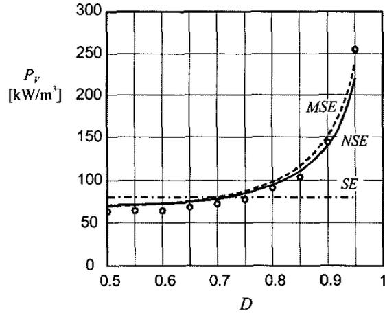
Fig.6 Specific ferrite core losses with square voltage waveforms for ferrite grade N67 at 100 kHz, 100°C, 0.1 T as a function of duty ratio  $D$ ; the experiments are the circles; the Natural Steinmetz Extension is the solid curve (NSE), for  $\alpha=1.76$ ;  $\beta=2.94$ ; the Modified Steinmetz Equation (5) is the dashed curve (MSE); classical Steinmetz Equation (1) is dash-dot curve (SE).
