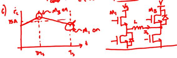
w) constant  $I_g$ .  $V_g$  tracks  $Q_g$  waveform under hard-switched conditions. When soft-switched, the "Miller plateau" will disappear. Because of direction of  $I_c$  & adequate  $t_{st}$ ,  $D_2$  &  $D_3$  are conducting during all turn-on transitions
