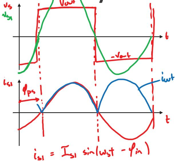
$$V_{out} = I_{out} R = \frac{2}{\pi} I_{s1} R \quad , \quad \text{by cap-Q balance on } C_f$$
