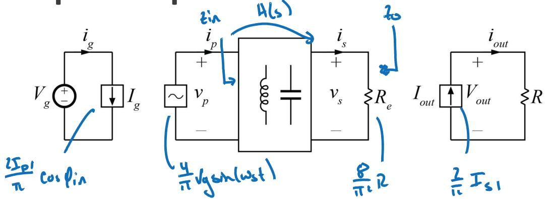
$\Phi_{in}$ ,  $I_{p1}$ ,  $I_{s1}$  determined by complete circuit
