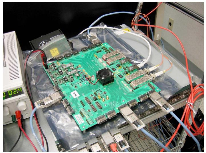
Fujitsu 20-port low-latency 10GbE switch being benchmarked in a Myricom lab
