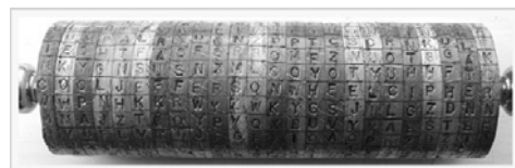
Jefferson cipher cylinder (36 discs, key is order of discs), 1790-1942 Adopted by US Army in 1922
