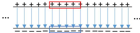
The electric field lines start from a positive charge and end at a negative charge.
