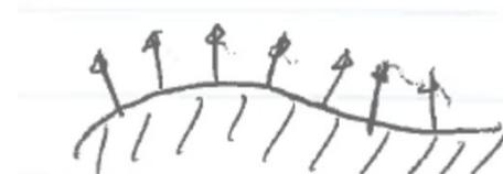
The electric field at a perfect conductor surface must be perpendicular to the surface.
