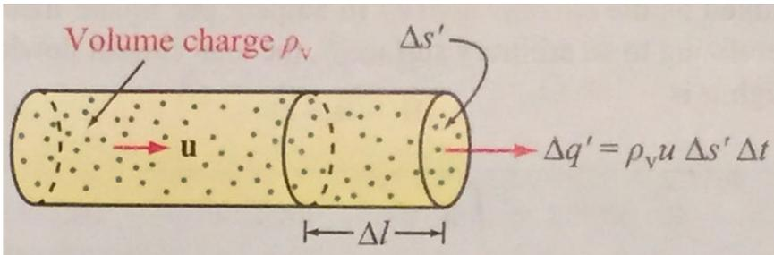
Conductor w/ **mobile** charge density  $\rho_v$ , or just  $\rho$  for short.
