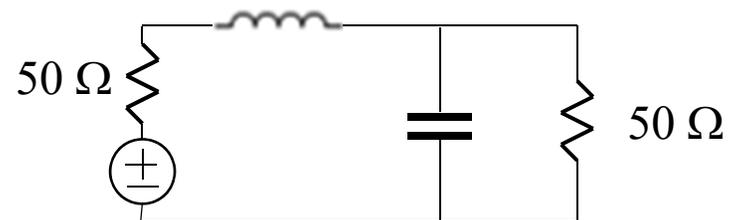
Generator: 1 V step, rise time = 0.1 ns. Internal impedance 50 Ω.
