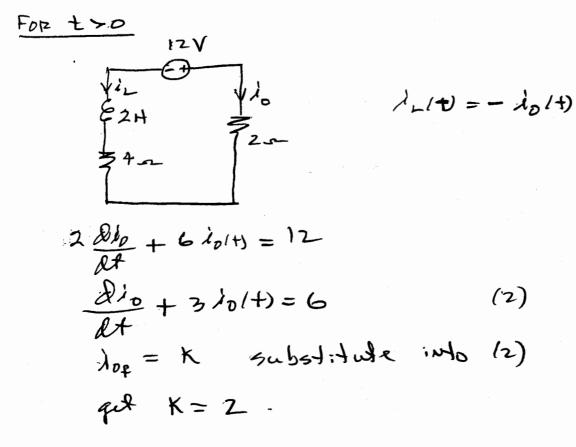
wig 6,23 Iont.  $i_0(t) = 2 + K_2 e^{-\frac{1}{T}}$ Ref = 65, L=2H 10(+) = 2+k2e^-3t iolot) = - is (o); runent through L cannot change inst. Go current through 22 is the negative of 1,10]. FROM (1) -1.2= 2+ K2 e-3t/+=0 -1,2=2+K2  $K_{2} = -3, 2$ 10(2)= 2-3.2 e A 220
