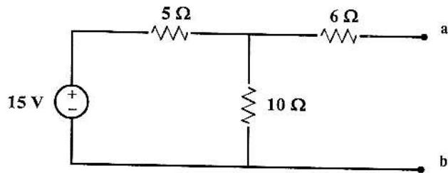
$$V_{ab} = \frac{15 \times 10}{10 + 5} = 10 \text{ V}$$
