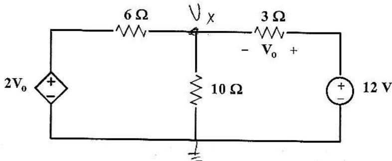
First use nodal; make  $V_x$  the unknown node voltage, write KCL at  $V_x$ .
