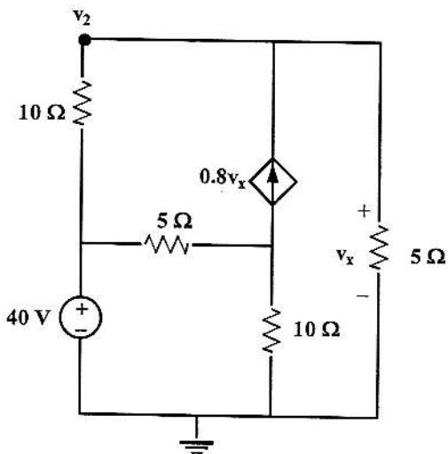
Write KCL using node  $v_2$
