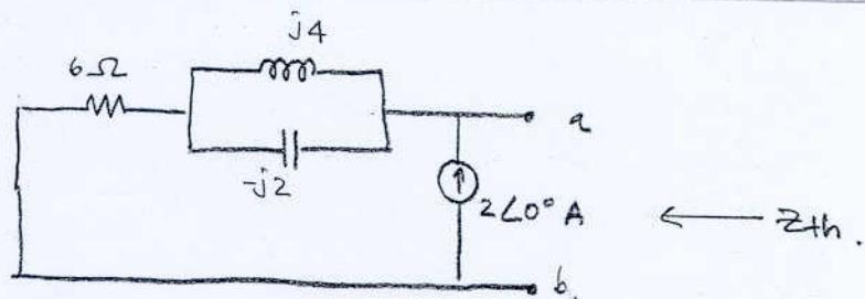
$$\begin{aligned} z_{TH} &= 6 + (j4// -j2) \\ &= 6 + \frac{(j4)(-j2)}{j4 - j2} \\ &= 6 + \frac{8}{j2} = 6 - j4 = 7.211 \angle -33.68^\circ \Omega \end{aligned}$$
