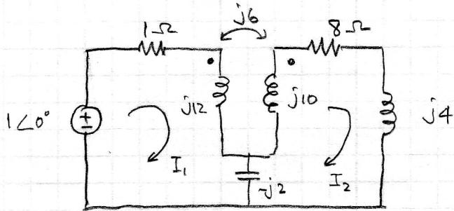
$$\text{Loop 1: } (1 + j12) I_1 - j_2 (I_1 - I_2) - j_6 I_2 = 1 \angle 0^\circ$$
