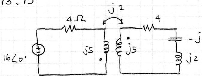
$$Z_{in} = Z_{\text{LEFT COIL}} + \frac{\omega^2}{Z_{\text{RIGHT COIL}}}$$
