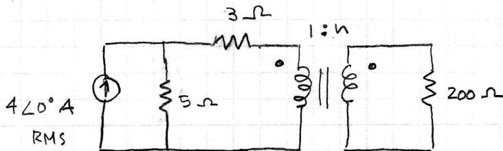
(a) FIND  $n$  FOR maximum power supplied to  $200\Omega$  LOAD.
