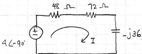
$$I = \frac{4\angle-90^\circ}{48 + 72 - j36} = \frac{4\angle-90^\circ}{120 - j36} = 0.03193 \angle -73.3^\circ$$
