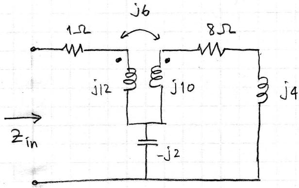
FIND the INPUT IMPEDANCE of the circuit.
