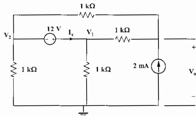
(4) Use nodal analysis to solve for  $V_o$  and  $I_x$  in the following circuit.  $V_o = 9 \text{ V}$ ,  $I_x = 3 \text{ mA}$
