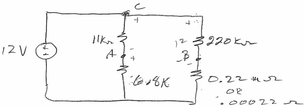
$$V_{CA} = \frac{12 \times 11K}{11K + 6.8K} = 7.416 \text{ V}$$
