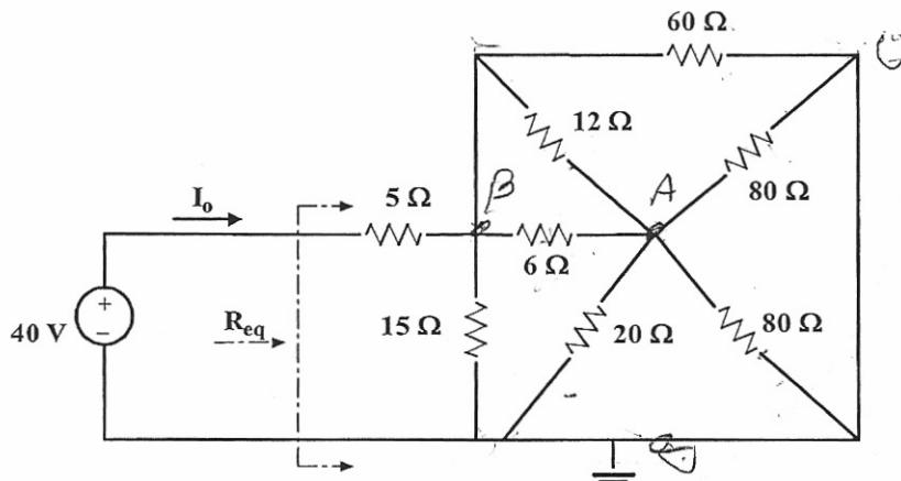
The  $6\Omega \neq 12\Omega$  are in parallel.  $G \parallel 12 = 4\Omega$
