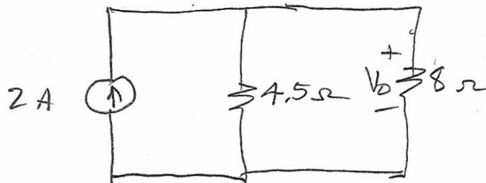
$$V_0 = \left( \frac{2 \times 4.5}{4.5 + 8} \right) 8 = 5.76 \text{ V}$$
