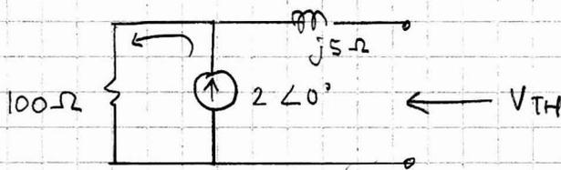
but there is no current flows through  $j5 \Omega$  due to open ckt, and there is zero voltage across  $j5 \Omega$ . Current from the current source only flows to  $100 \Omega$ .
