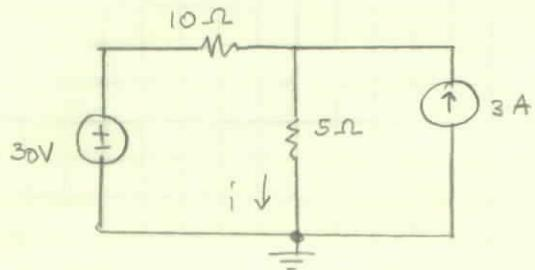
Find  $i$  using superposition principle.
