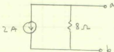
This verify that  $i_{sc} = I_N = -2A = -\frac{16V}{8\Omega} = \frac{V_{TH}}{R_{TH}}$ .
