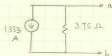
We verify that  $i_{sc} = I_N = -1.333 A = \frac{-5V}{3.75\Omega} = \frac{V_{TH}}{R_{TH}}$
