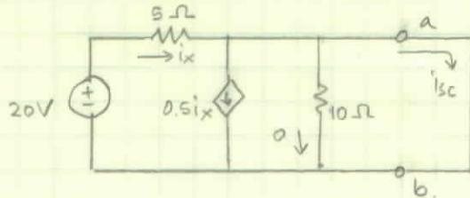
$$ix = \frac{20 \text{ V}}{5\Omega} = 4 \text{ A} \rightarrow Isc = ix - 0.5ix \\ = 0.5ix \\ = \underline{\underline{2 \text{ A}}}$$
