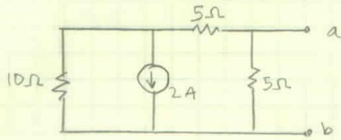
FIND the max. power that can be delivered to a RESISTIVE LOAD by the circuit.
