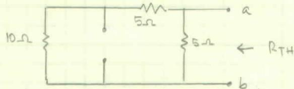
$$R_{TH} = (10+5)\parallel 5 = 15\parallel 5 = \frac{15 \times 5}{15+5} = \frac{75}{20} = 3.75\Omega$$
