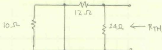
$$\begin{aligned} R_{TH} &= 12 // 24 \\ &= \frac{12 \times 24}{12 + 24} = 8\ \Omega = R_{TH} \end{aligned}$$
