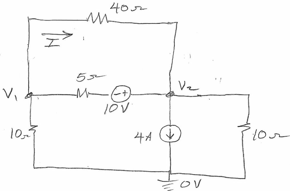
Use nodal analysis to find  $V_1$ ,  $V_2$  and  $I$ .
