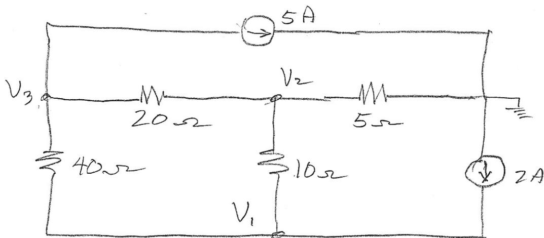
We could just as well use  $V_1$  as ground and relabel the remaining nodes.
