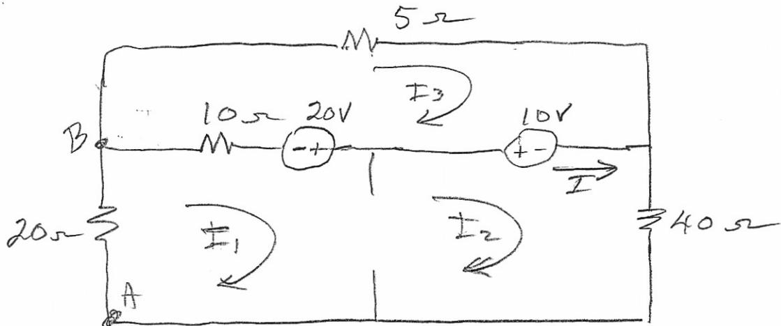
We still retain the identity of  $I_1$ ,  $I_2$ , and  $I_3$ . In the above circuit we have 2 closed paths. We write KVL around these paths. This gives 2 equations.
