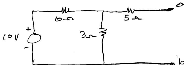
$$V_{ab} = V_{os} = V_{TH} = \frac{10 \times 3}{9} = \frac{30}{9} = \frac{10}{3} V$$
