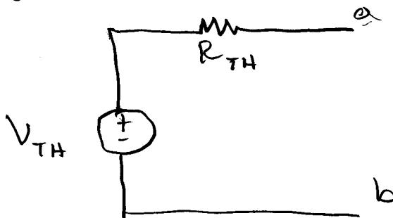
After all, if you placed a voltmeter across a-b you would read a voltage: This is the "open-circuit" voltage.
