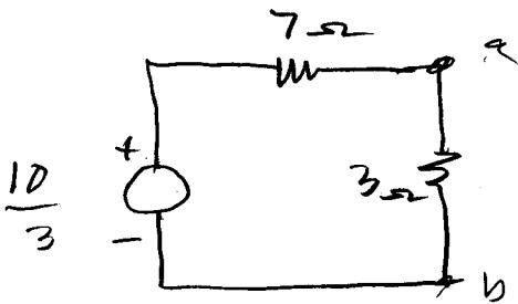
$$V_{ab} = \frac{\left(\frac{10}{3}\right) \times 3}{7+3} = 1V$$
