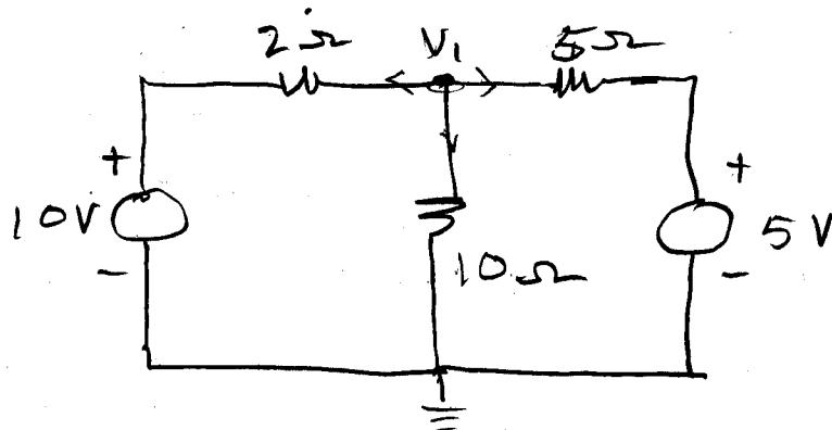
Find  $V_1$  using superposition;
