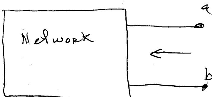
Suppose we have only resistors and sources (voltage and/or current sources).
