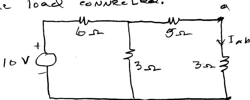
Remove the load. Find  $V_{os}$ .
