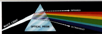
Plan 1. Color spectrum seen by passing white light through a prism. (Courtesy of General Electric Co., Lamp Business Division.)
