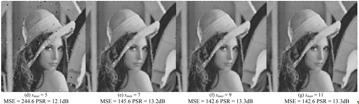
Fig. 6. The first row contains images showing the blurring and noising process. The second row shows results from adaptive median filtering.
