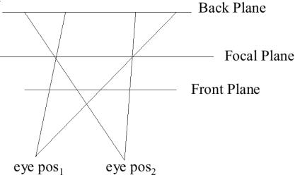
Move the camera in a plane parallel to the focal plane.
