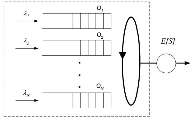
**Figure 1.** A basic model of the virtual input queueing architecture at an egress port of an output queued switch. Each logical queue corresponds to a different input port.
