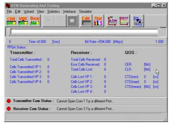
Figure 3. ATM analyzer software user interface
