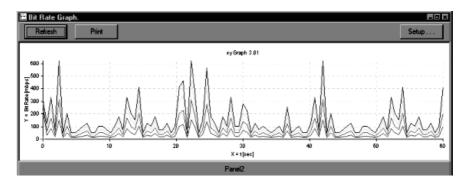
Figure 4. Example of synthesized traffic; instantaneous bit-rate (Mbit/sec) versus time for four different destinations
