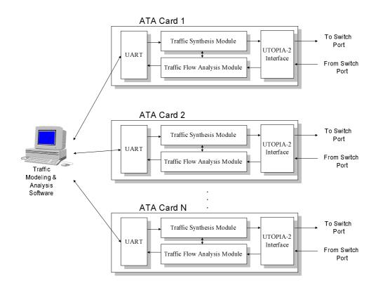
Figure 1: ATM Analyzer System Layout
