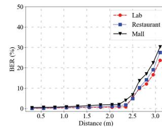
Figure 13: BER of room-scale system under different environments.
