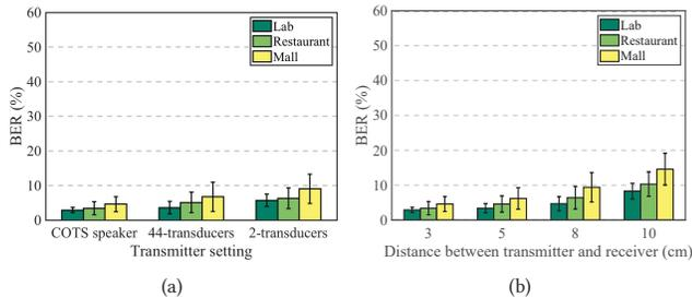
**Figure 9: BER of BatComm under different (a) transmitter settings and environments (b) distances between transmitter and receiver (Throughput = 34.13kbps).**
