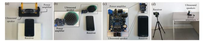
Figure 8: Illustration of four experimental settings with different types and numbers of ultrasound speakers (power cables are not included). (a) COTS ultrasound speaker (Vifa); (b) Customized 44-transducer array; (c) Customized 2-transducer array; and (d) Two ultrasound speakers for room-scale communication.
