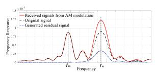
Figure 3: Illustration of the signals on the subcarrier  $f_n$  affected by the residual signal (e.g.,  $f_n = 2f_m$ ).
