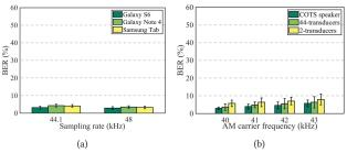
Figure 12: BER of BatComm under different (a) sampling rates and receiver devices (b) AM carrier frequencies.
