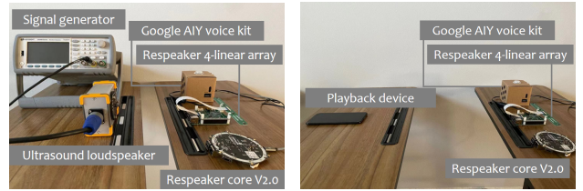
(a) Setup for inaudible attack (b) Setup for the remaining audio attacks
