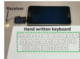
Fig. 9. Experimental setup of localizing touches: keystroke recognition on a paper keyboard.
