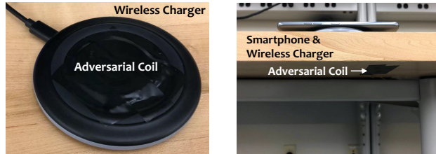
(a) Stealthily sticking an ultra-thin adversarial coil on the surface of the charger (b) Hiding the adversarial coil underneath the surface
