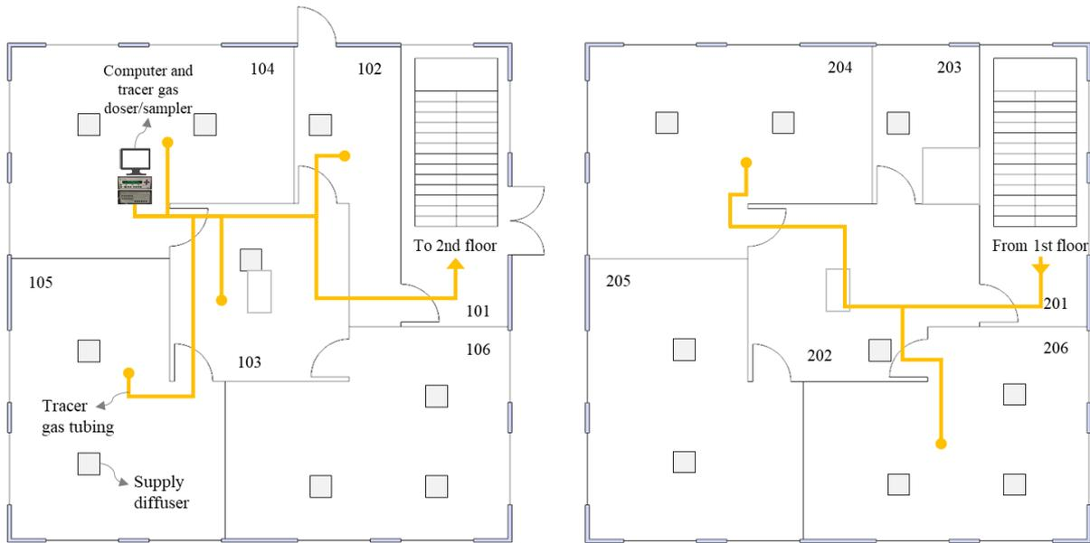
Figure 4. Test set: multichannel doser and sampler.
