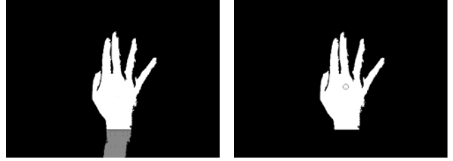
Figure 6. Image before and after threshold is applied to remove the arm; the circle was added only to enhance the location of the refined centroid.
