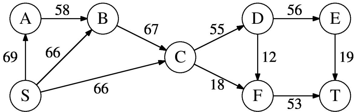
Part 1: Helen is using the Edmonds-Karp algorithm for determining the maximum network flow from S to T in this graph. Specify the first augmenting path (Do this by listing the nodes in order in a single string, like SABCDEFG).
