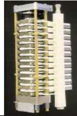
IGBT (Transistor) Valve HVDC Light
