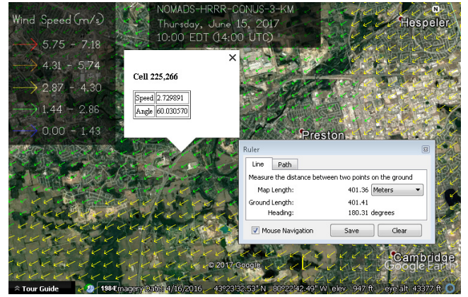
Fig. 17. Zoom-in view of downscaled wind data. The balloon shows the wind speed and direction of the selected data point. The ruler tool shows that the spatial resolution of downscaled wind data is about 400m (~1300ft).
