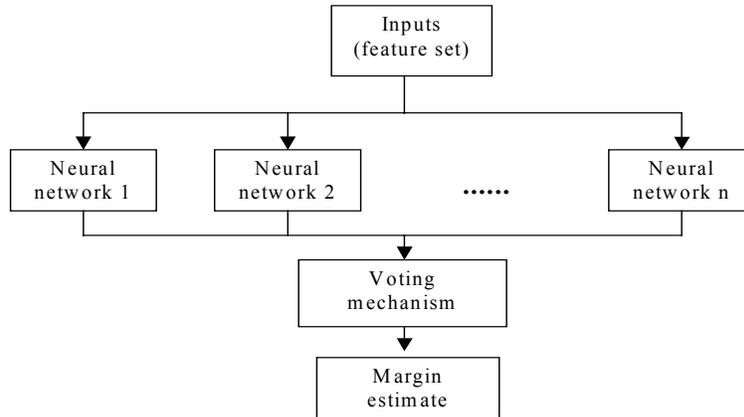
Fig. 3 Individual estimators with voting mechanism
