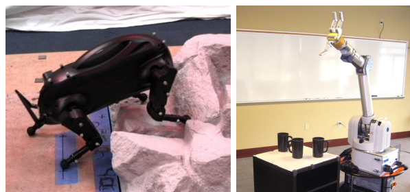
Fig. 1. Experimental robotic platforms: Boston Dynamics’s LittleDog (left), and Barrett Technology’s WAM arm (right).
