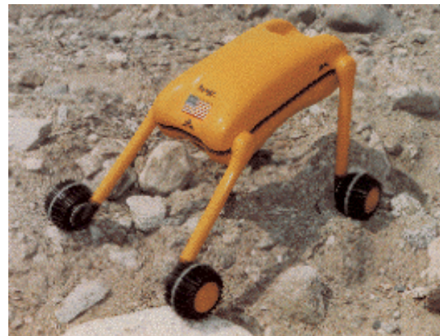
Gofer, with active center of gravity compensation
