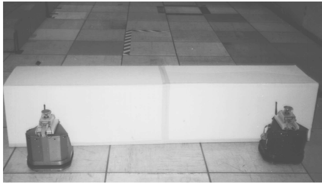
Fig. 5. The beginning of the box pushing application. Two R-2s are pushing the box across the room. (The R-2 robot GREEN is on the left, the R-2 robot BLUE is on the right.)
