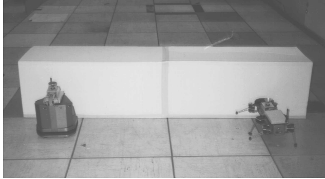
Fig. 8. Adaptivity due to heterogeneity. In the second experiment, we again seize one of the R-2 robots, but this time we replace it with GENGHIS . Since GENGHIS cannot push as powerfully as an R-2, the remaining R-2 robot adapts its actions by pushing less frequently.
