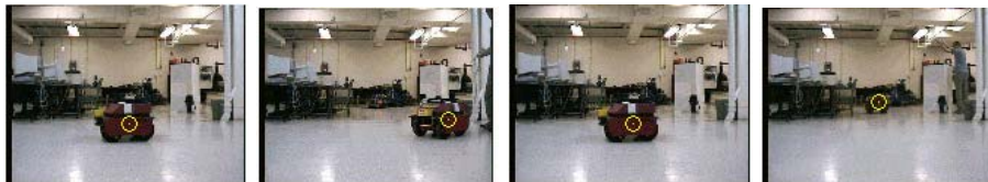
Fig. 3. Results of visual tracking approach. Small white circles indicate locations of robots detected by the visual tracking algorithm.
