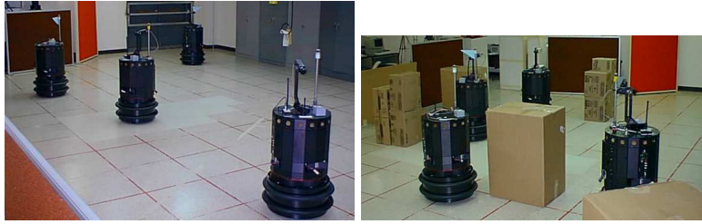
Fig. 2. Robot team executing hand-generated solution to CMOMMT. The first photo shows robots operating in an area with no obstacles. The second photo shows the robots amidst randomly distributed obstacles.
