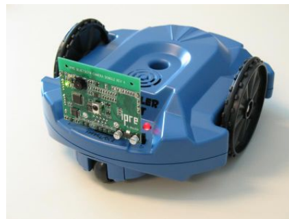
Figure 1: The Parallax Scribbler with IPRE Fluke attached. This is the hardware configuration supported by both Myro and Myro-C++. The Scribbler+Fluke combination is sold for about $200 at the time of writing. (Photo courtesy of IPRE)
